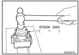
3. Install flow control valve A, flow control valve spring and flow control valve B assembly to locations shown in the figure.
