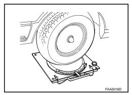
Start engine and run at idle, turn steering wheel all the way right and left, measure the turning angle.
