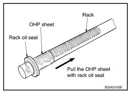
b. Insert rack oil seal (inner) to piston (rack Teflon ring) position and push retainer to adjust screw side with fingers lightly, and then make rack move in gear housing assembly, install rack oil seal (inner) to fit with gear housing assembly.
