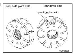
8. Install vane to rotor with facing the round portion outside.
