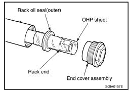
5. Using a 45 mm (1.77 in) open head (suitable tool), tighten end cover assembly at the specified torque.
