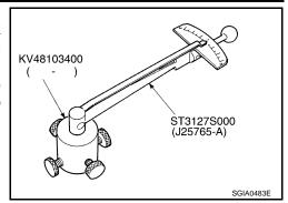
15. Measure pinion rotating torque with torque adapter (SST) and preload gauge (SST), then confirm whether it's reading is within the specified value. If the reading is not within the specified value, readjust screw angle with adjusting screw. Change gear assembly to new one, if the reading is still not within the specified value or the rotating torque of adjusting screw is less than 5 N⋅m (0.51 kg-m, 44 in-lb).
