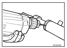
10. Remove end cover assembly with a 45 mm (1.77 in) open head (suitable tool).
