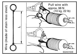
c. Twist boot clamp as shown in the figure, pay attention to relationship between winding and twisting directions.
