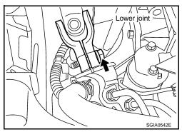
10. Remove mounting bolts of steering gear assembly with power tool, and then remove steering gear assembly from vehicle.
