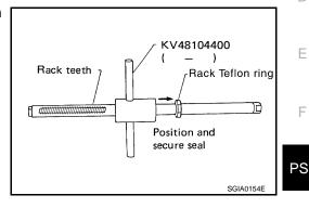
Apply recommended grease to rack oil seal. Insert rack oil seal, then insert rack assembly to gear housing assembly.
