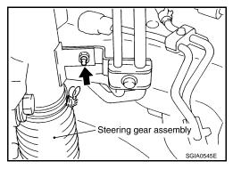
9. Remove mounting bolt (lower side) of lower joint.
