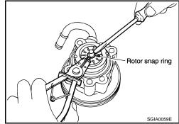
Remove cam ring, rotor, vane, front side plate, flow control valve
