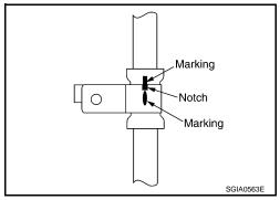
To install eye joint, join projection of eye joint into notch of power steering pump, and attach eye joint to power steering pump properly. Then, tighten eye bolt by hands fully, and tighten it with a specified torque.
