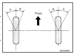
Measure rack stroke if angles are outside the specified value.
