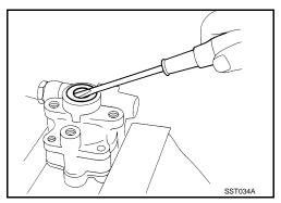
Loosen lock nut and remove washer, O-ring, joint then remove connector bolt, O-ring and pull out flow control valve and spring from body assembly.
