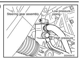
8. Remove mounting bolt of steering hydraulic piping bracket from steering gear assembly.
