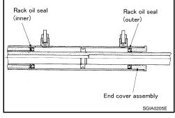
a. To avoid damaging inner rack oil seal, wrap an OHP sheet [approximately. 70 mm (2.76 in)  $\times$  100 mm (3.94 in) around rack tooth. Place oil seal on sheet. Then, pull oil seal along with OHP sheet until they pass the toothed section of rack, then remove it.
